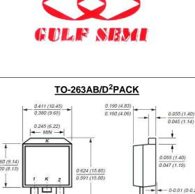
0.360 (9.14) 0.320 (8.13) 0-0.01 (0-0.254) 0.110 (2.79) 0.027 (0.686) 0.021 (0.53) PIN 1 O 0.037 (0.940) 0.014 (0.36) -0 K - HEATSINK PIN 2 O 0.105 (2.67) 0.140 (3.56) 0.095 (2.41) 0.110 (2.79) 0.205 (5.20) 0.195 (4.95) Dimensions in inches and (millimeters)
